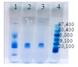
Fig.1. Cylindrical Gel Electrophoresis (SDS Polyacrylamide) pattern of Coot egg white and Hen egg white RfBPs 1.Coot egg white crude 2.Coot egg white G-100 eluted fraction 3.Hen egg white G-100 eluted fraction 4.Rtotein Molecular weight marker(20.100to97.400 Kd.)
