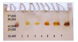
Eig. 5. Siliver staining on SDS Polyacrylamide Cel Electrophoresis pattern of Coot egg white and yolk RfBPs U.Protein molecular weight marker (18,400 to 97,000Kd) U.Coot egg white DEAE Sepharose eluted fraction U.Coot egg white Sephadex G-100 fraction U.Coot egg yolk Sephadex G-100 fraction U.Coot egg yolk DEAE Sepharose eluted fraction U.Coot egg yolk DEAE Sepharose eluted fraction U.Coot egg yolk DEAE Sepharose eluted fraction U.Hen egg yolk Sephadex G-100 U.Hen egg yolk Sephadex G-100
